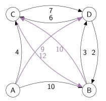
Step 3.1: Contract the loop (B-C) into one node, and create a new graph.
