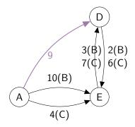
Step 3.2: Contract the loop (B-C) into one node, and create a new graph, with the adjusted weights.
